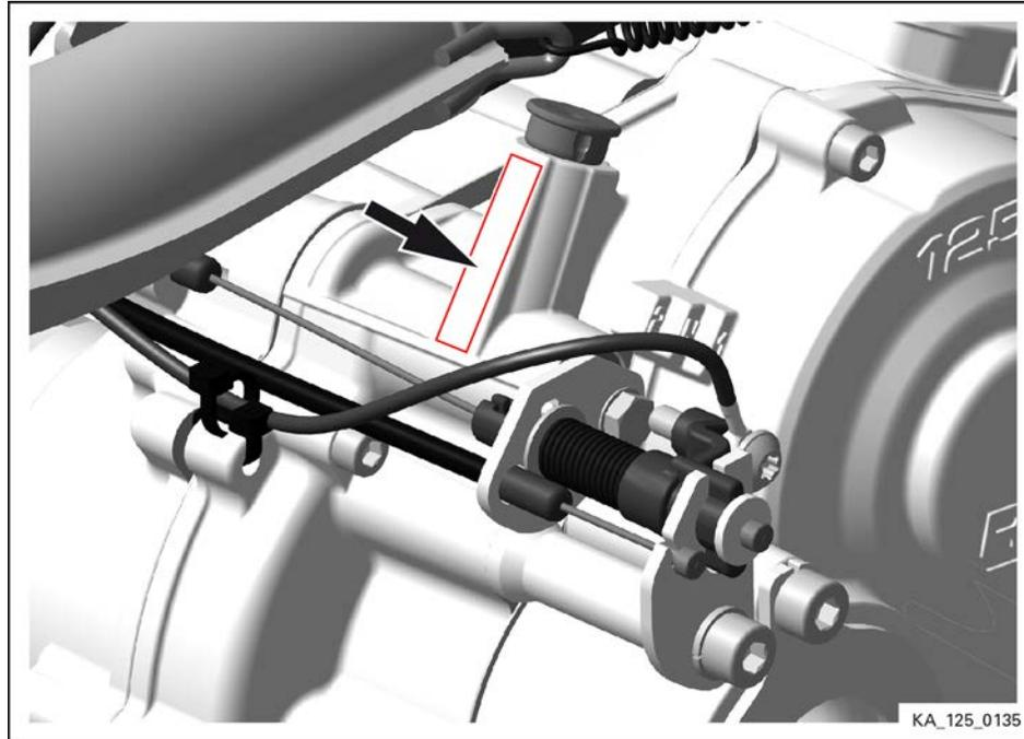
Figure 1.4: Serial number of the engine, TYPICAL
