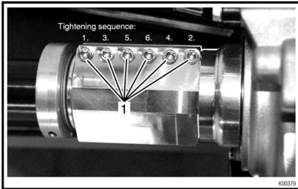
Figure 2.4: Tightening sequence
