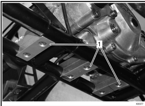
Figure 2.3: Engine brackets
