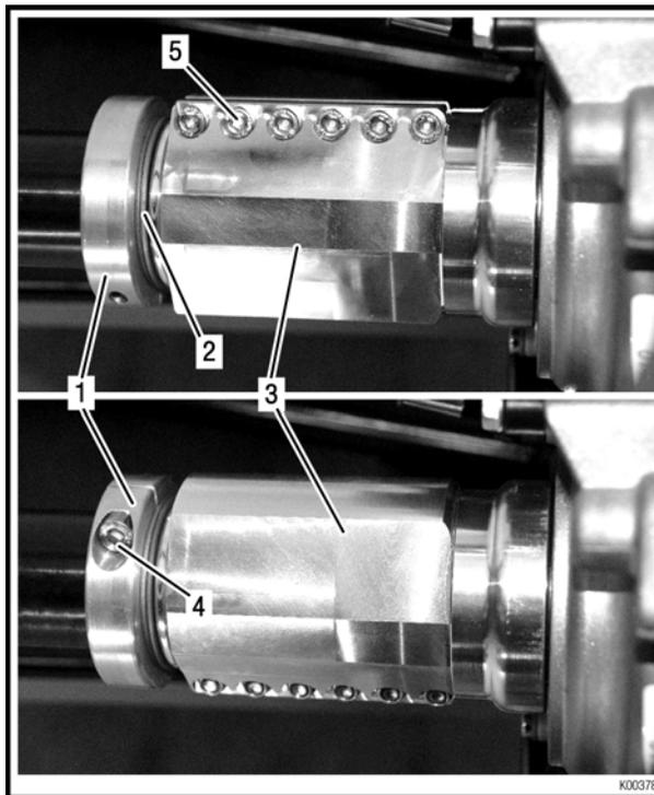
Figure 2.2: Overload clutch
